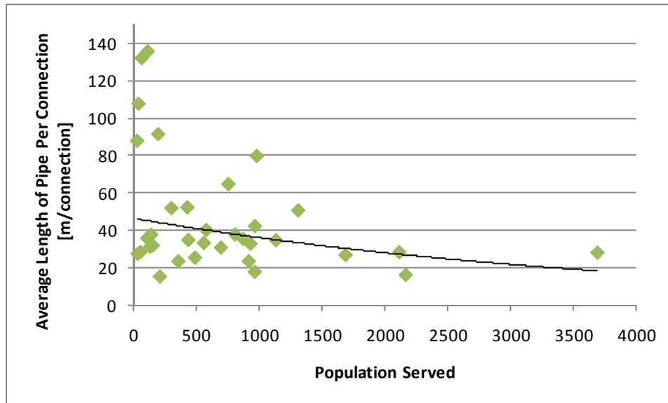
**Figure 3.3 - Wastewater Collection - Average Pipe Length per Connection**
